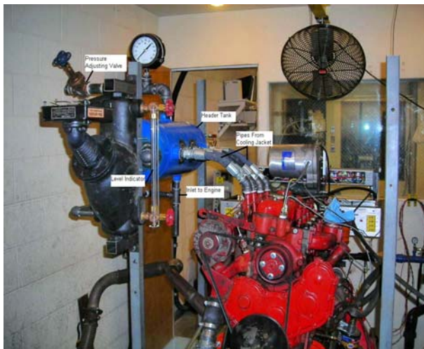
Figure 4. Engine test setup on the dynamometer
