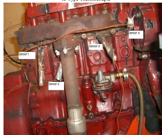
Figure 5. Thermocouples installed in the cylinder head
